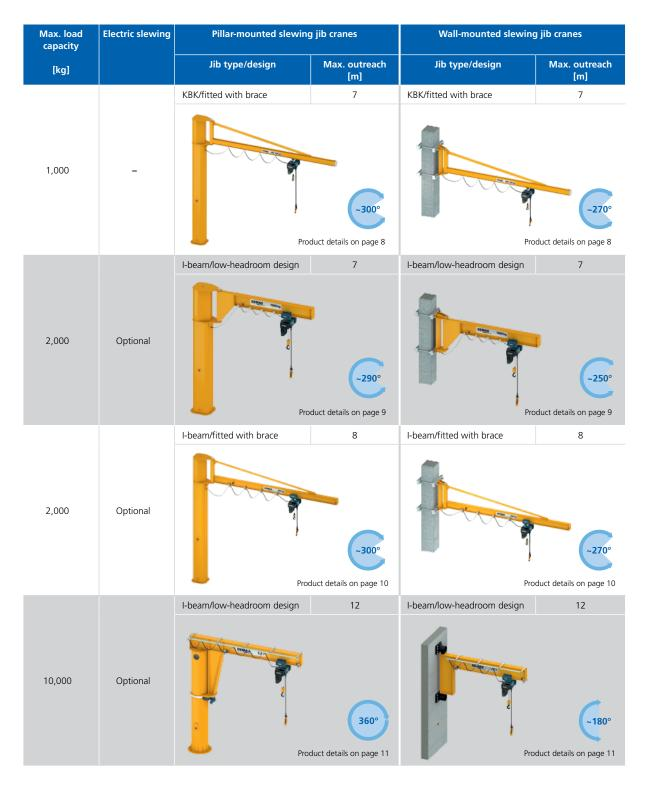
The crane types shown on the following pages are designed for indoor operation as standard. The surfaces of steel superstructure components are coated to meet the requirements of corrosivity category C2M.
