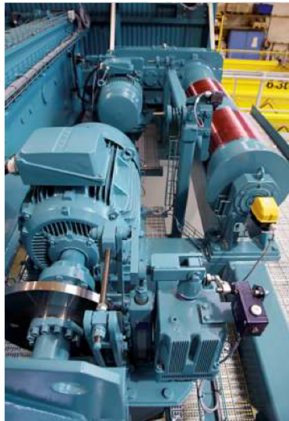
6E - Open winch with double planetary gearbox double drum and safety brake drum
