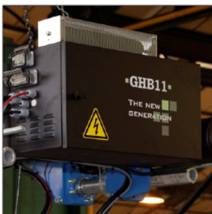
17 Hoist electric cabinet
